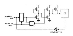
FIGURE 3. QUASI-BIDIRECTIONAL PORT STRUCTURE
